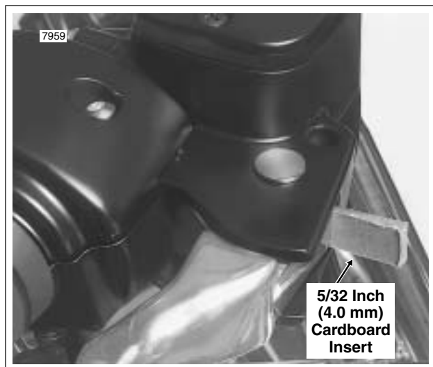
Figure 2-153. Install Cardboard Insert
