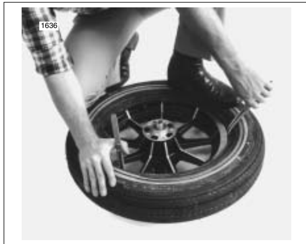
Figure 2-32. Starting Second Bead on Rim
