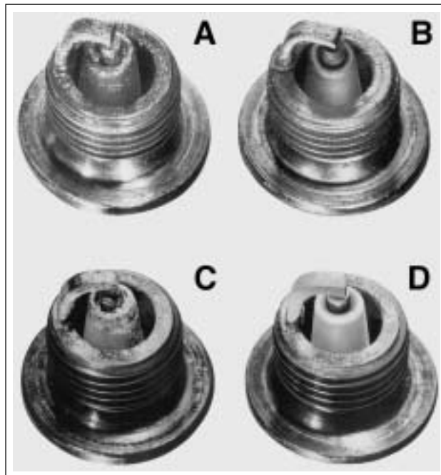
Figure 8-9. Types of Plug Base Deposits
