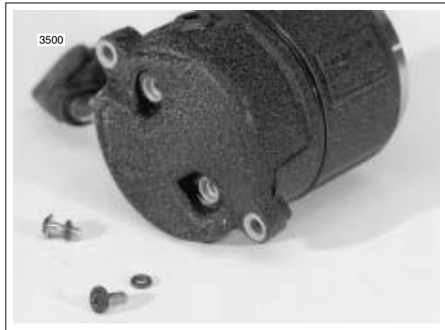
Figure 5-7. Remove End Cap Screws and O-Rings
