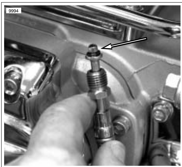
Figure 2-23. Clutch Fluid Line O-ring
