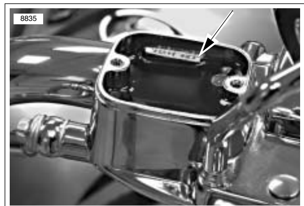
Figure 1-2. Fill Level (reservoir cover removed as viewed from front of motorcycle)
