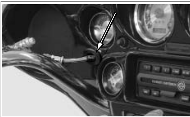
Figure 2-24. Clutch Fluid Line Inner Fairing Grommet
