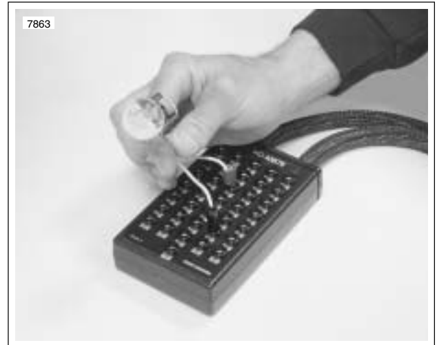
Figure 4-31. Ignition Coil Circuit Test
