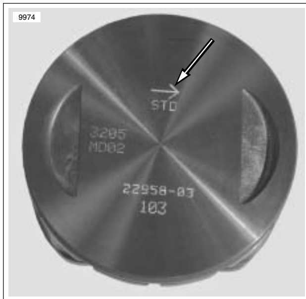
Figure 3-7. FLHTCSE Piston Orientation Arrow (arrow points to front of engine)
