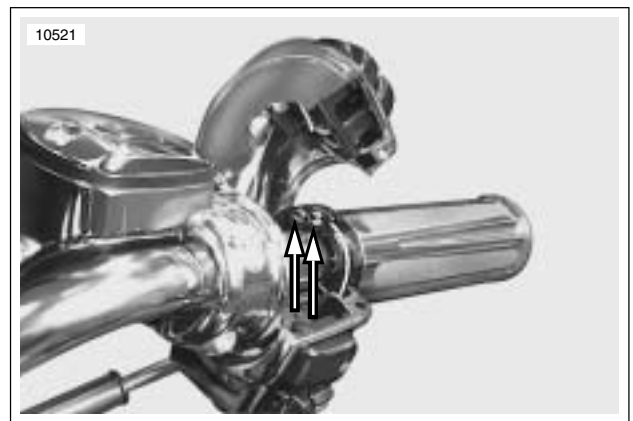
Figure 2-14. Throttle and Idle Cable Ferrules
