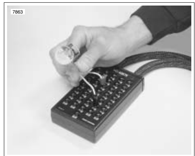
Figure 5-17. Ignition Coil Circuit Test
