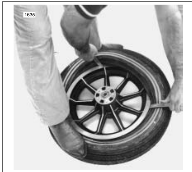
Figure 2-31. Starting Bead on Rim
