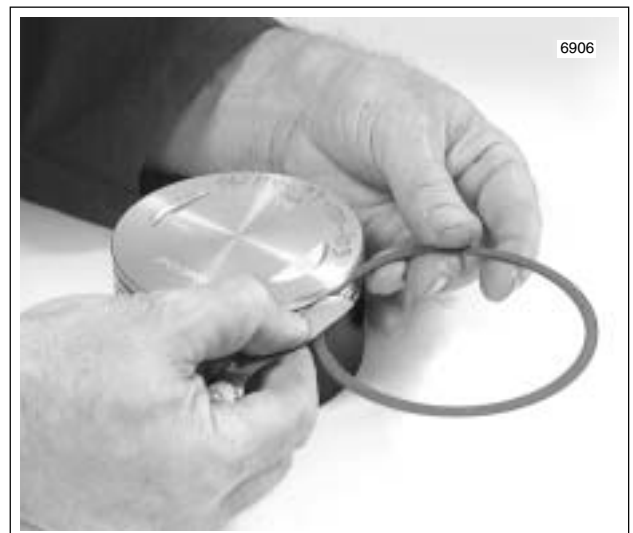
Figure 3-88. Measure Piston Ring Side Clearance
