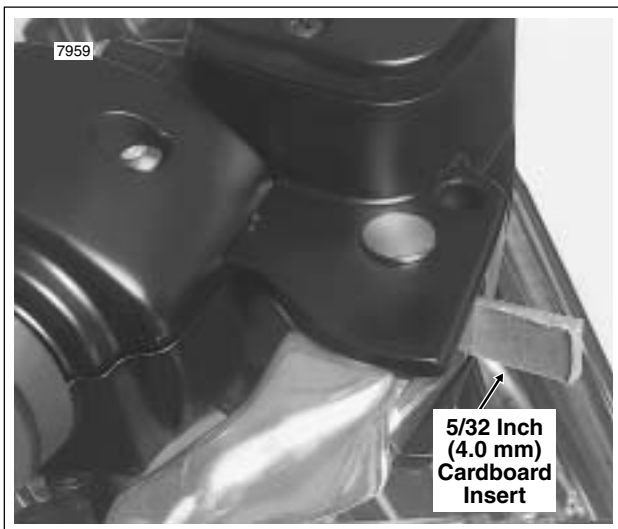
Figure 2-41. Install Cardboard Insert Before Removing Master Cylinder Assembly
