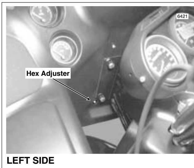
Figure 8-32. Headlamp Adjustment (FLTR)
