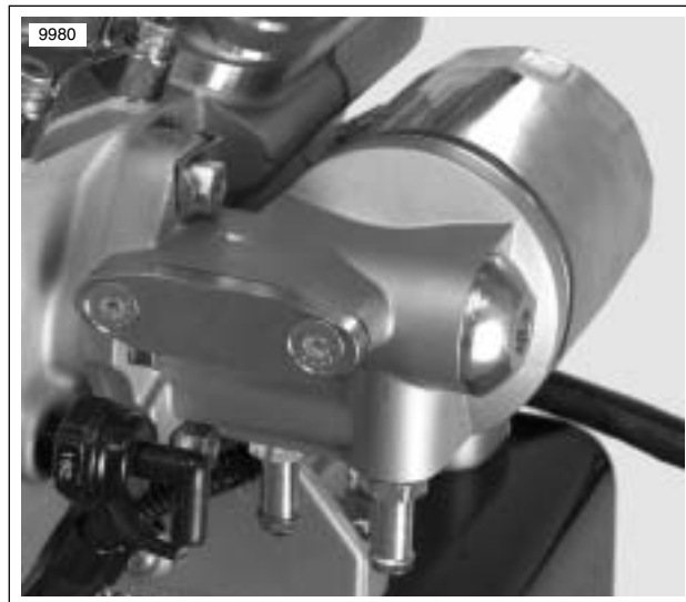
Figure 3-25. Oil Filter Mount (engine removed from frame)
