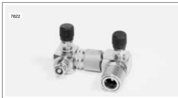
Figure 5-32. Fuel Pressure Gauge Adapters
