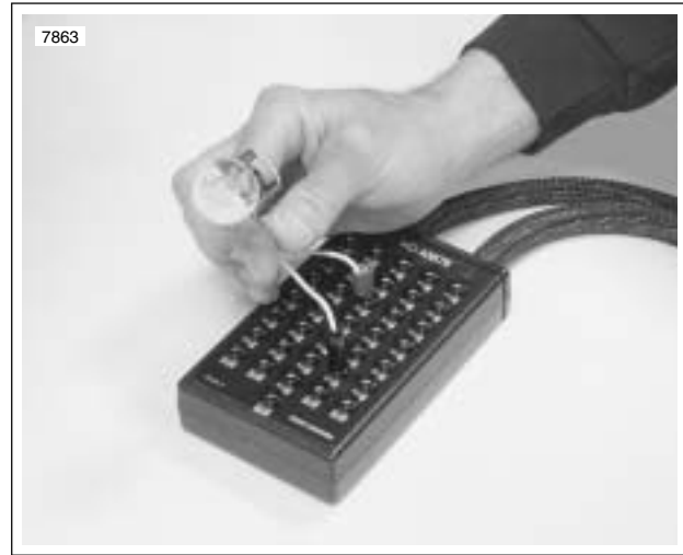
Figure 5-67. Ignition Coil Circuit Test
