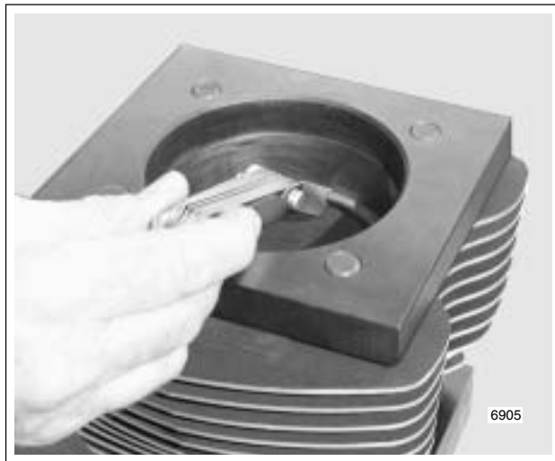
Figure 3-91. Measure Ring End Gap
