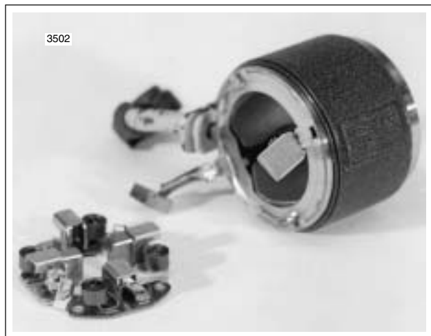
Figure 5-9. Remove Brush Holder
