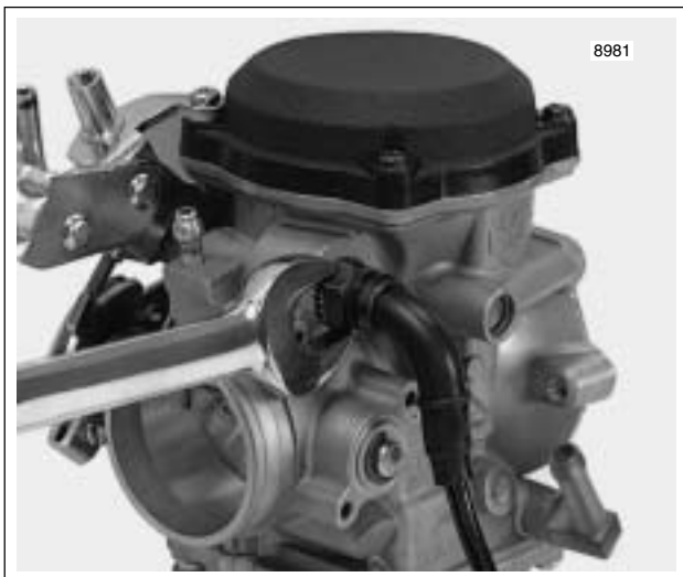
Figure 4-6. Remove Enrichener Cable
