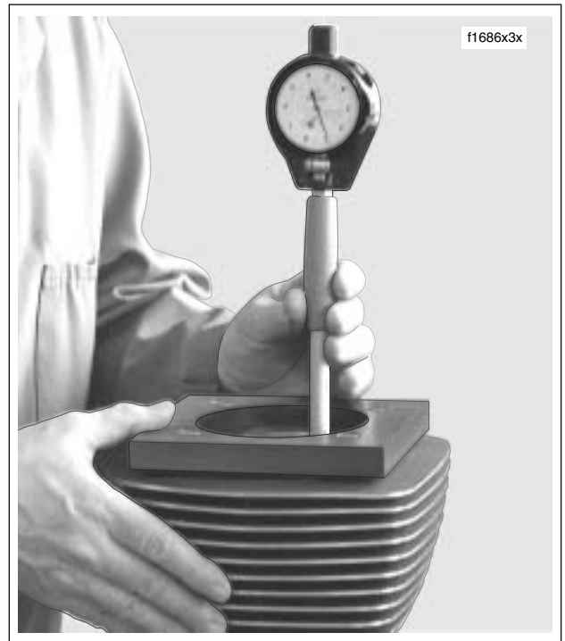
Figure 3-87. Measure for Out-of-Round and Taper
