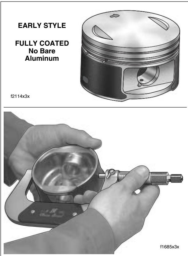
Figure 3-89. Measure Early Style Piston for Running Clearance
