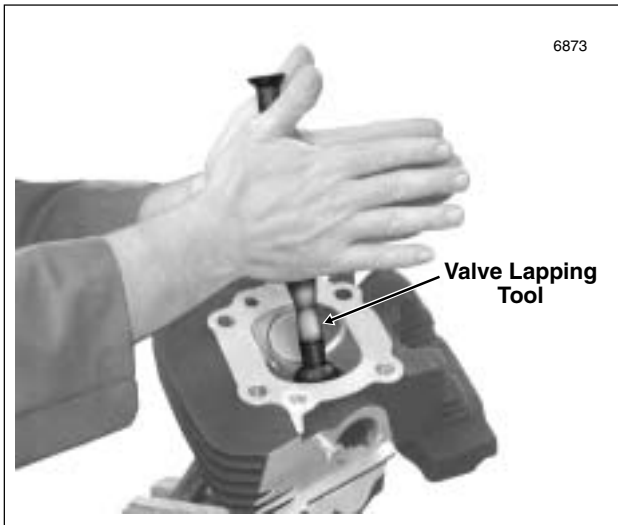
Figure 3-80. Oscillate Tool to Create Contact Area
