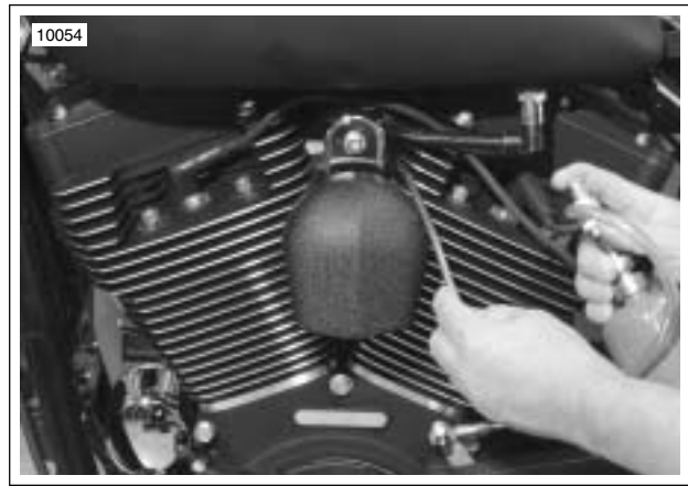
Figure 5-15. Checking for Leaks
