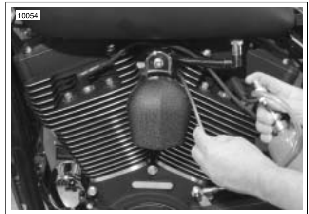
Figure 4-14. Checking for Leaks
