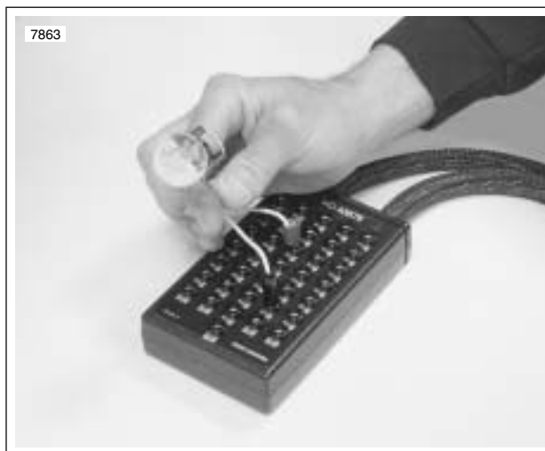
Figure 4-16. Ignition Coil Circuit Test
