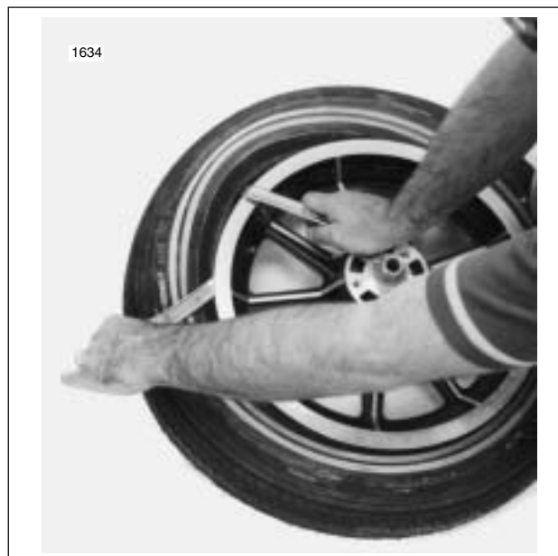
Figure 2-29. Starting Bead Off Rim
