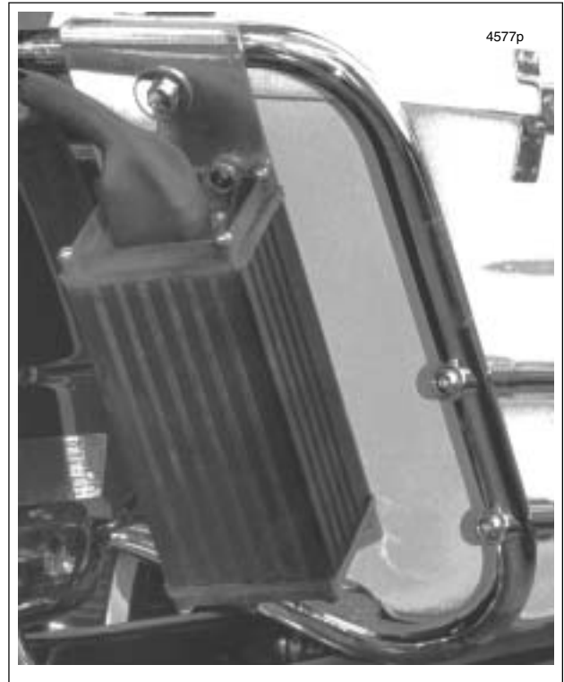
Figure 8-26. Whelen Amplifier Mounting
